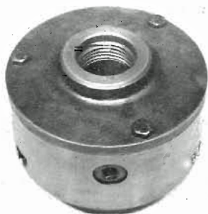
Fig. 75 Chuck with Backplate attached
