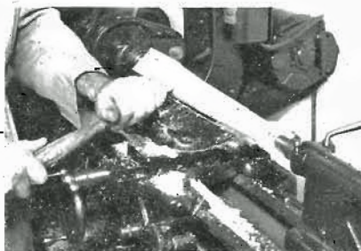
Fig. 174 Wood Turning Between Spur and Cup Centres
