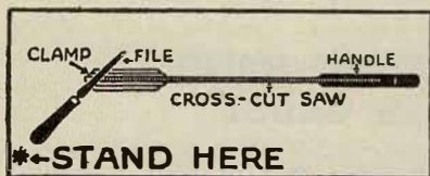
Fig. 10 — First position for filing handsaws for cross cutting.
