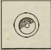
Fig. 14 Drill slides off-centre
