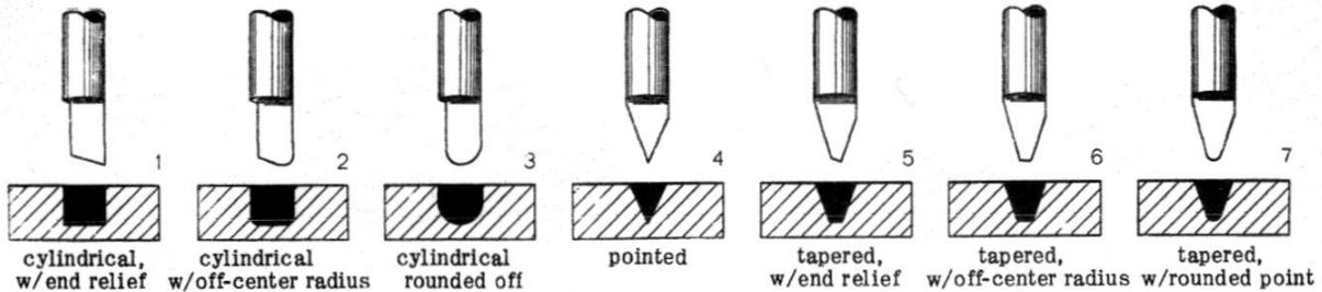
Above are illustrated the seven basic cutter profiles and cross-sectional views of the profiles they will produce.
