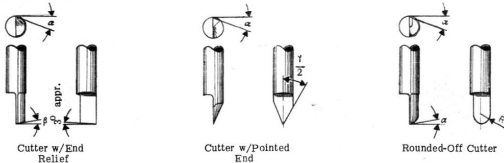
Angle  $\beta$  applies for end relieved cutters only. Cutters having an angle  $\alpha$  of less than  $20^\circ$  should be relief ground at between  $25^\circ$  and  $30^\circ$  (see special instructions).
