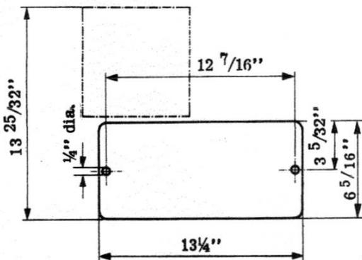
**Chucking and Grinding Capacity**
