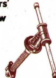
The screw and handle are of the best mild steel with stub Acme thread. Attention is drawn to the particularly sturdy fittings and the strong full-circle thrust flange on the nut.
